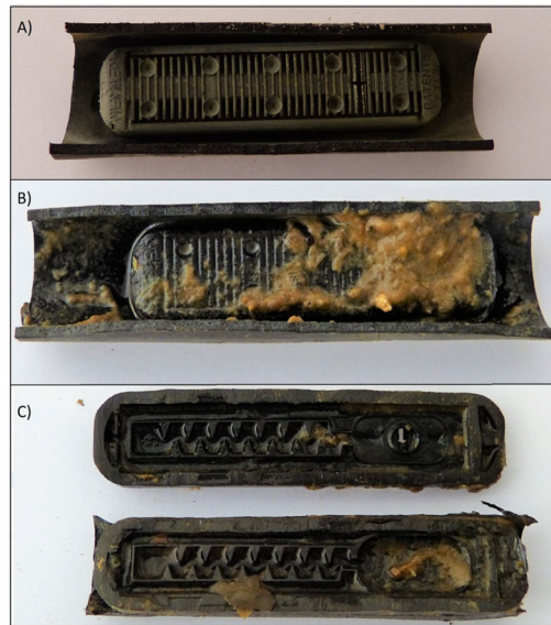
Figure 7. External views of an emitter protected by the porous media underdrain filter placed at the first location (A) at last location (B), and inside view of the last one (C) after 1000 h of irrigation.
