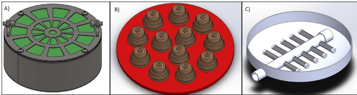
Figure 1. Different underdrain designs: porous media (A), inserted domes (B) and arm collector (C).
