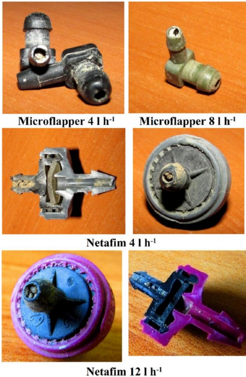
Figure 4. Samples of clogging of Microflapper and Netafim emitters
