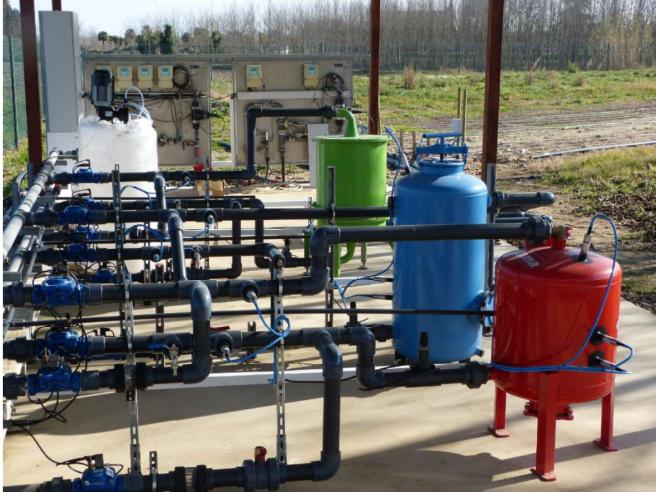
Fig. 1. Picture of the experimental set-up with the three filter designs: (a) red: arm collector; (b) blue: inserted domes; and (c) green: porous media prototype.
