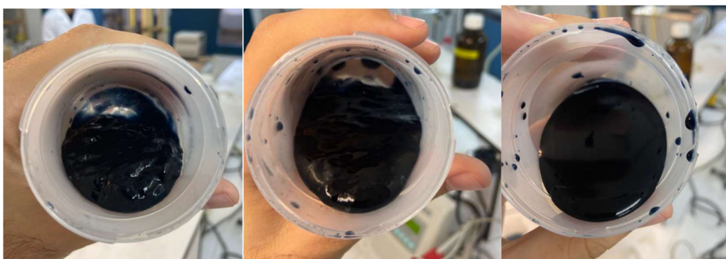
Figure 29. 70-30 / 50-50 / 30-70 (in order left to right) conductive hydrogels after 4 days drying by casting.
