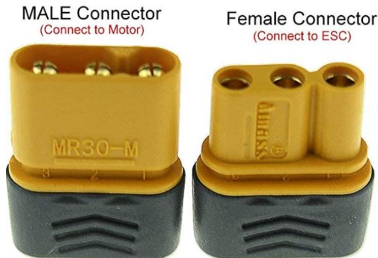
Figura 52. Connectors MR30 per a connectar motors i controladors.
