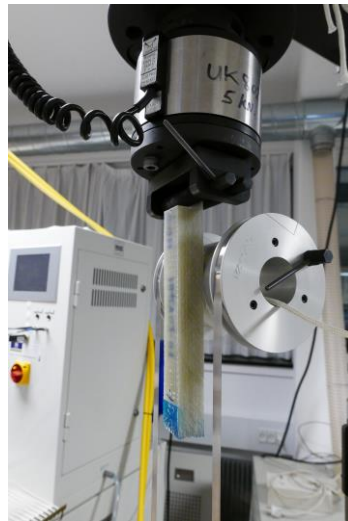
Figure 1: Climbing drum peel test setup
