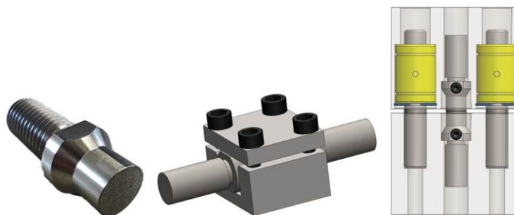
Figure 2: Left: Isometric real view of the BJ bonnet specimen. Middle: render of the adherent-bar mounting system. Right: Render of the BJ manufacturing tooling system.
