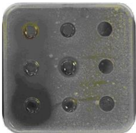
Figure S1. Photography of the tetracyclines Water-Scan plate with the nine wells, four of them showed inhibition zone (the three on the left and the one in the center), whereas the others did not show inhibition.
