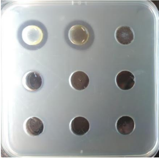
Figure S2. detail of an inhibition plate with the 9 wells. The two upper left wells presenting an inhibition growth area.
