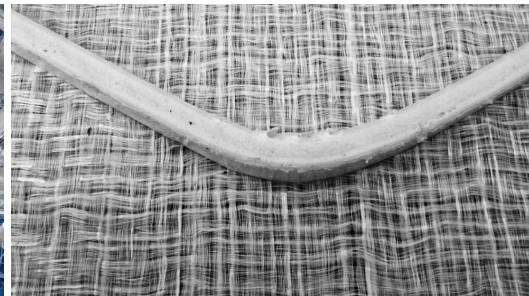
(d) A foamed composite panel flexed and stressed.
