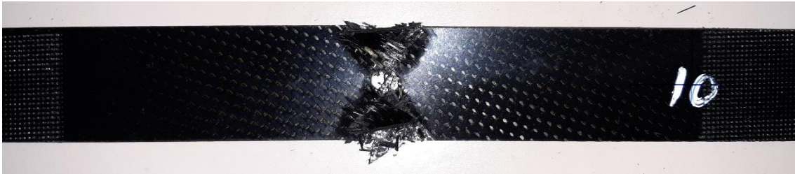
Figure 6.12. AIR-3R failed specimen under OHT test
