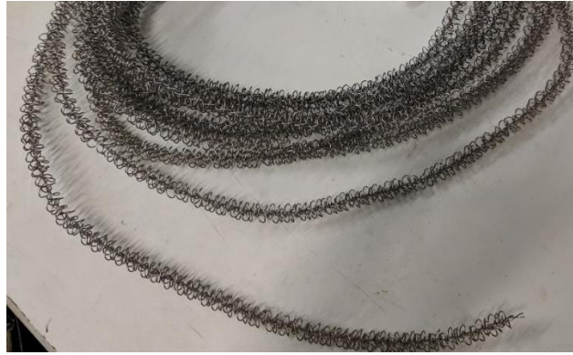
Figure 4.18. Metal mesh used to improve the mixture between the resin and hardener inside the machine injection nozzle.
