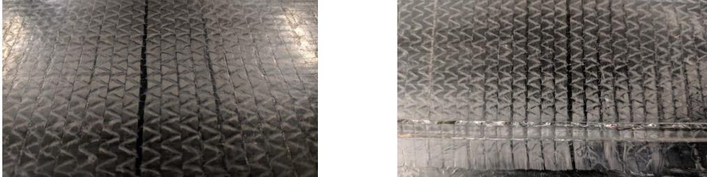
Figure 5.5. Process defects related to preform handling
