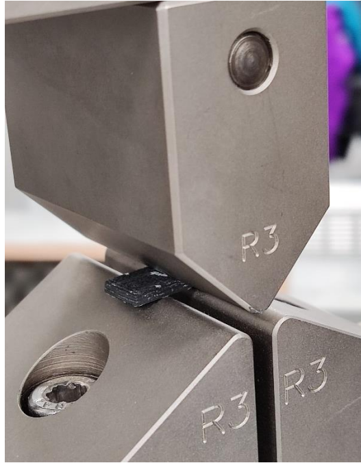
Figure 3.16. Positioning of ILSS coupons for testing
