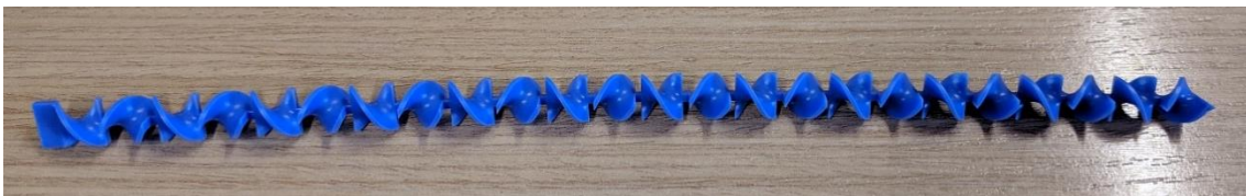
Figure 4.19. Commercially available static mixer. Dimensions are the same as the injection nozzle cavity, material is compatible with the operative temperatures.
