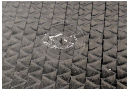
Figure 5.31. Superficial defect found at the sample injected at 8 MPa and 80° C. Close up to the local defect at the sensor location
