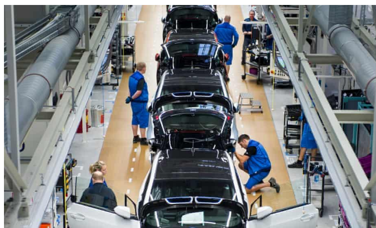
Figure 1.1. Building line for the BMW i3, a passenger car with a carbon fiber structure. [15]
