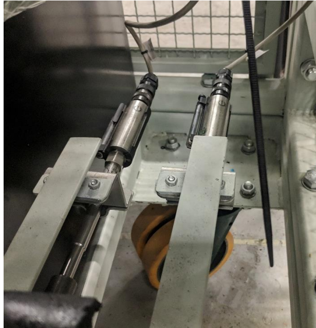
Figure 4.13. Resin (left) and hardener (right) pressure sensors. Pressure for the injection lines
