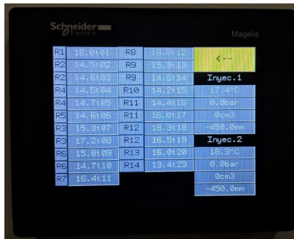
Figure 4.12. Machine heating monitoring and resin and hardener parameters control (pressure, flux and current position)
