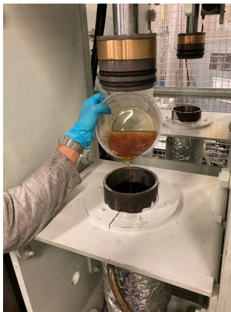
Figure 3.6. Pouring of the resin mixture inside the injection tanks.
