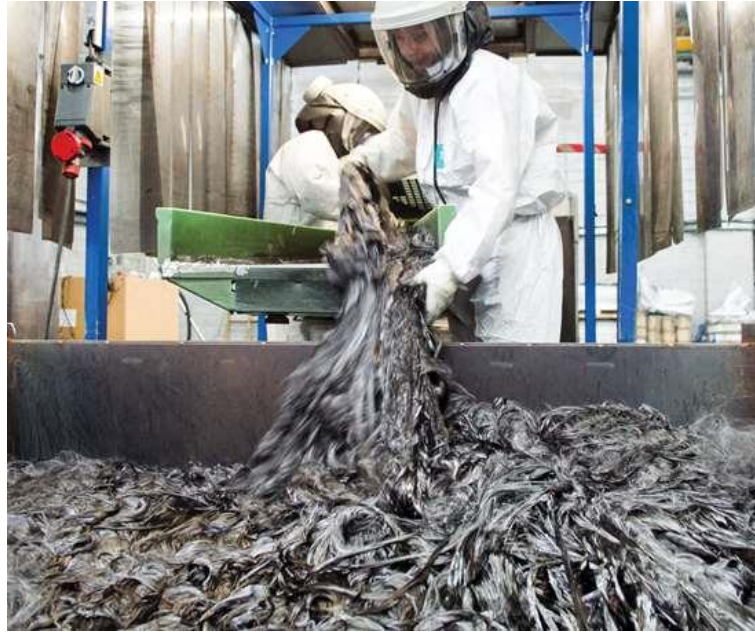
Figure 1.2. Reclaiming of carbon fiber by pyrolysis in composite waste. [30]
