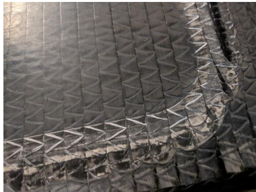
Figure 5.9. Detail of a dry zone under the clamping area for the trial injected with an O-ring with bigger diameter than the intended by design
