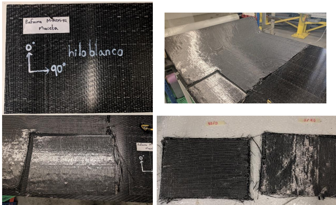
Figure 3.4. Cutting of individual fabric layers using the plastic template and the defined reference directions
