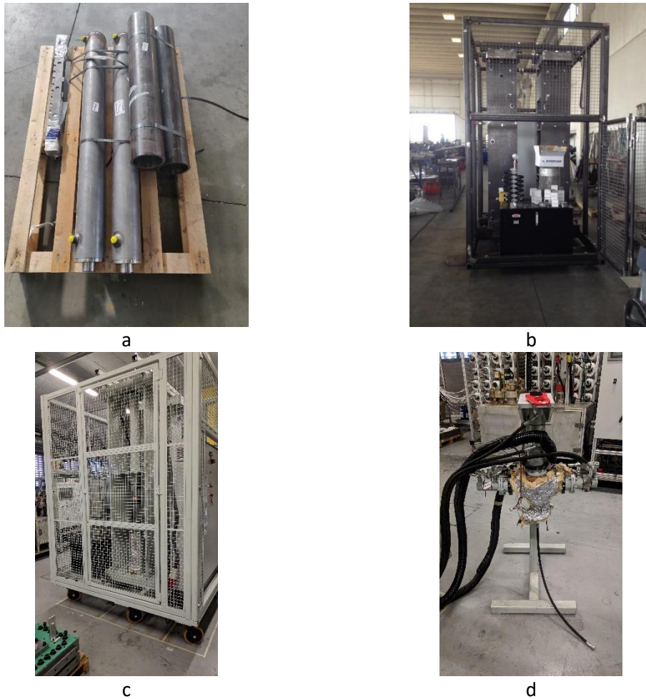
Figure 4.2. Machine construction and final assembly (Courtesy of MSX Tech.) (a) Axial pistons array and machine resin and hardener tanks. (b) Main machine frame with support plates (vertical) for the axial pistons and hydraulic array (pump and oil tank). (c) Final enclosure of the machine with security doors (lateral view axial pistons and electric panel). (d) Mixhead with dosing pistons (laterals), resin hoses and hydraulic connections (attached to the machine frame).
