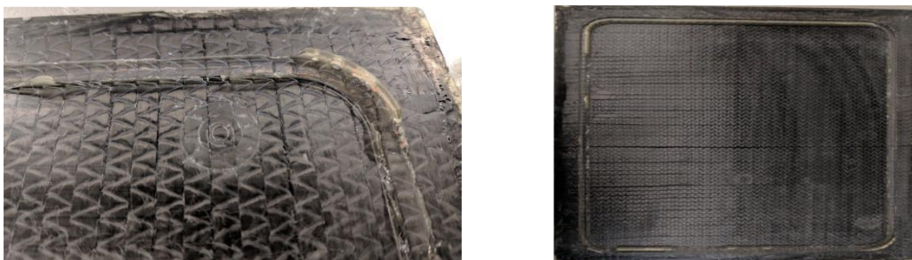
Figure 5.4. Visible superficial marks on the composite sample made by the sensors and the fiber clamping mechanism
