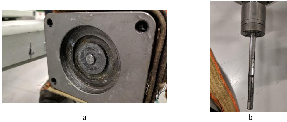
Figure 4.22. Failure of the cleaning piston. a) Stuck piston in the closed position inside the mixhead core. b) Piston after removal with the solidified O-ring
