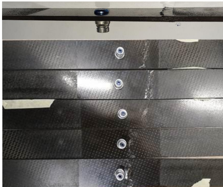
Figure 6.15. Failed FHC specimens
