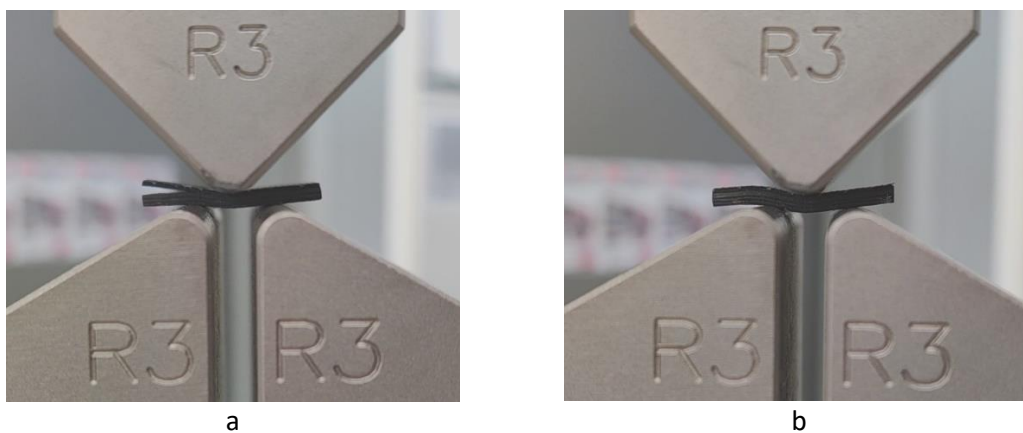
Figure 5.21. Examples of ILSS failures. a) Interlaminar shear failure. b) Plastic failure
