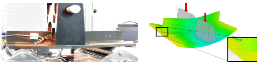
Figure 3: Technological sample testing: 3 points bending experiment and model.
