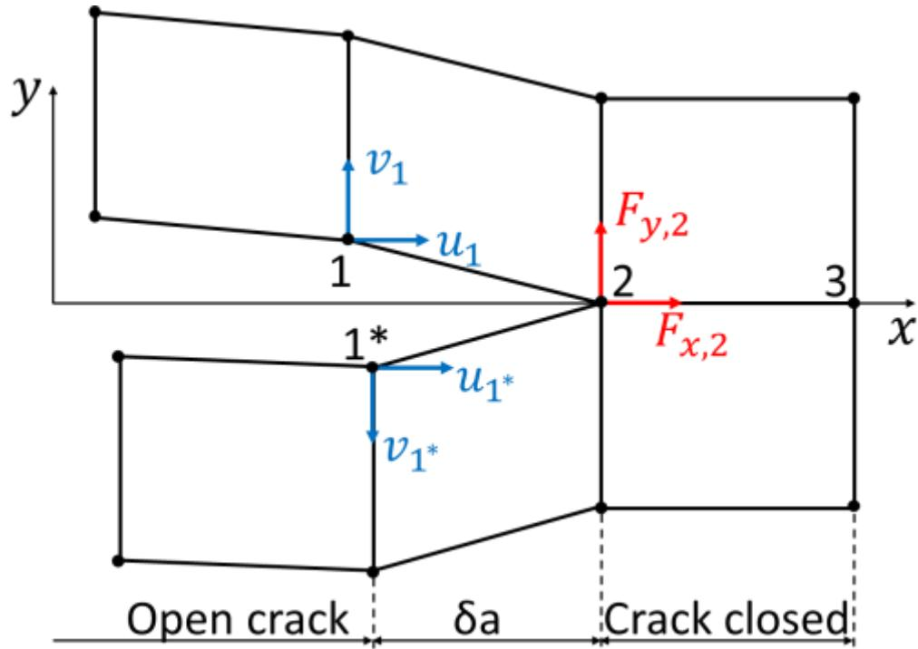
Strain Energy Release Rate computation technique
