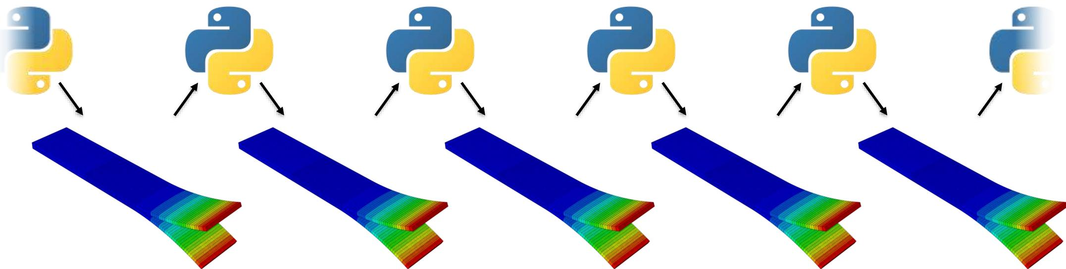
Fatigue load history is simulated via a series of static simulations
