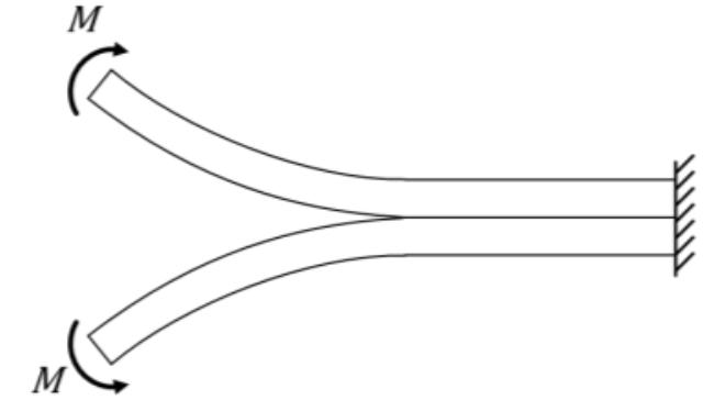
$$\frac{da}{dN} = f \left( g_{\max}, g_{\min}, \frac{g_{II} + g_{III}}{g_{tot}} \right)$$
