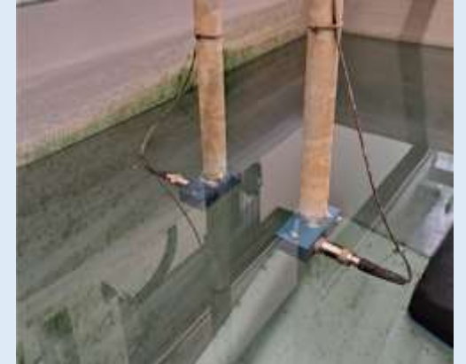
Through thickness transmission ultrasound scan
