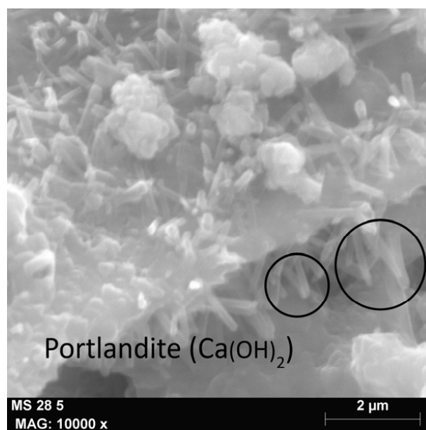
Figure 8. SEM images of portlandite at 28 days, \times 10,000 in a mortar without fibers.
