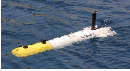
Fig. 6. Sparus II AUV, a nonholonomic vehicle.
