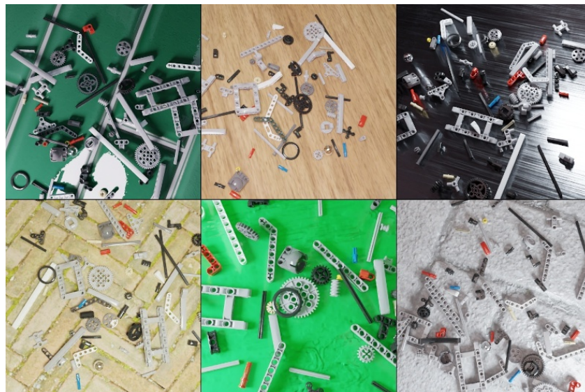
Figure 5. Synthetic dataset, showing synthetically generated images with different backgrounds and camera and light positions.
