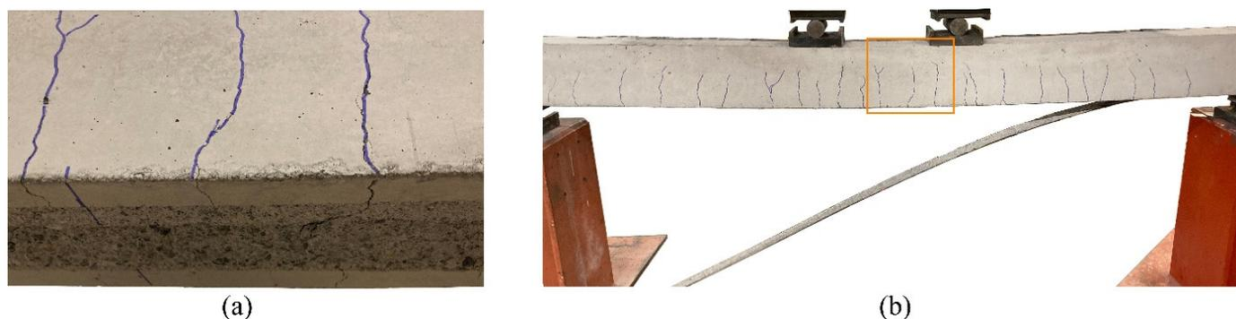
**Figure 6.** Failure of beam EBR-I-d10: (a) Failure surface and (b) ICD failure and crack pattern.
