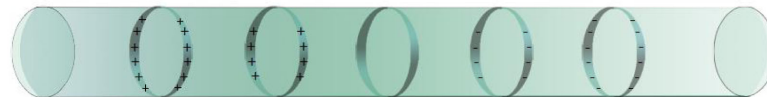
Figure 2: excess of electrons is on the surface of the conducting wire. Which of the students is right? Why?
