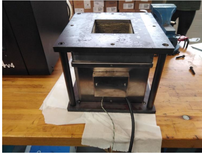
Figura 42: Part estructural subjectant la part calefactors
