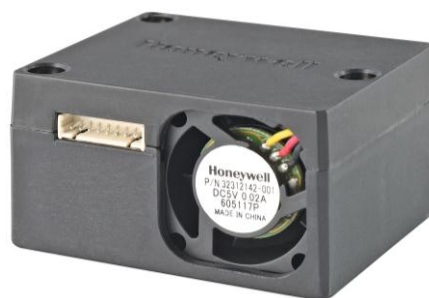
Figura 24: Sensor Honeywell HPMA115S0
