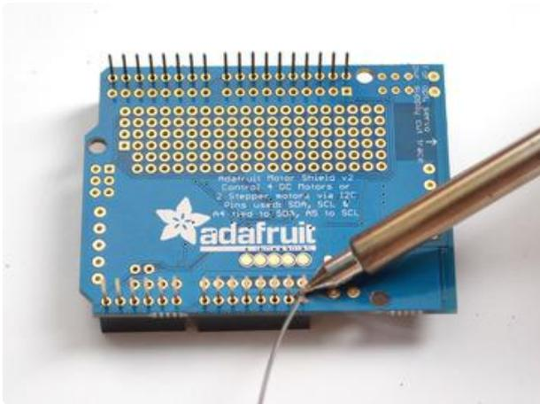
Tack one pin of each header, to get them set in place before more soldering. If the headers go crooked you can re-heat the one pin while re-positioning to straighten them up
