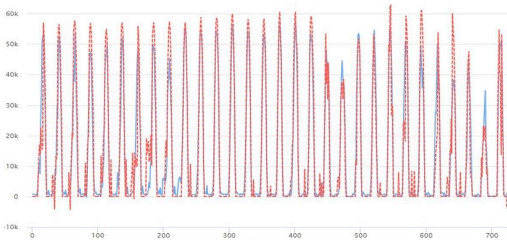
Fig. 4. PV generation forecasting. On vertical axis there is the PV generation (blue) and the PV generation prediction (red) in Watts. In horizontal axis there is the time in hours.
