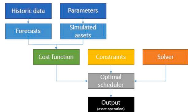
Fig. 1. Block diagram of the inputs and outputs of the OS.
