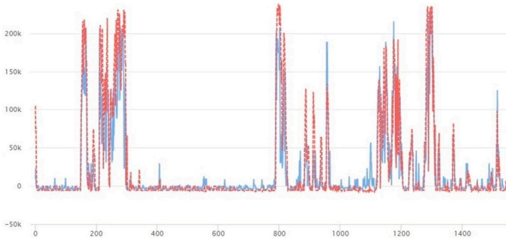
Fig. 5. WT generation forecasting. On vertical axis there is the WT generation (blue) and the WT generation prediction (red) in Watts. In horizontal axis there is the time in hours.
