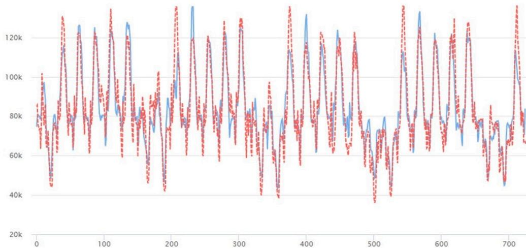
Fig. 6. Non-controllable consumption forecasting. On vertical axis there is the non-controllable consumption (blue) and the non-controllable consumption prediction (red) in Watts. In horizontal axis there is the time in hours.
