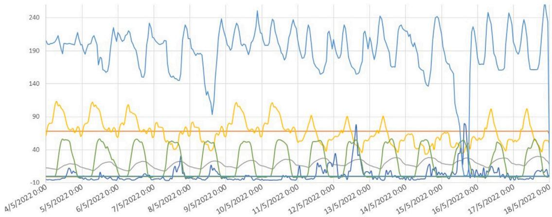
Fig. 8. OS inputs for each of the 14 days. In vertical axis there is the electricity selling price in euros/MWh (orange), the building consumption in kW (yellow), the solar production in kW (green), the outdoor forecasted temperature in Celsius (grey), the wind production in kW (dark blue) and the electricity buying price in euros/MWh (blue). In the horizontal axis there is the time in hours.
