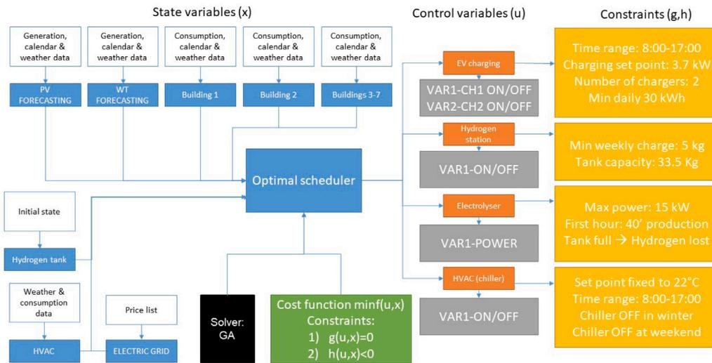
Fig. 3. Walqa pilot block diagram of the OS.
