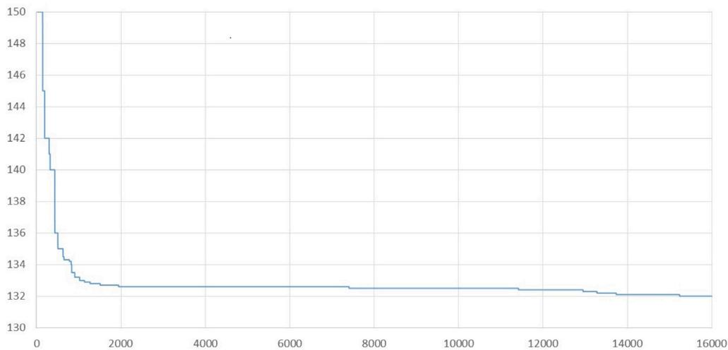
Fig. 11. Cost function evolution for one specific day. Vertical axis is the cost of the best solution in the actual population expressed in euros. Horizontal axis are the iterations.
