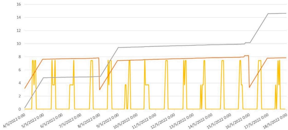
Fig. 9. Simulation of assets over the experimentation period. In vertical axis there is the tank profile in kg (orange), EV chargers consumption in kW (yellow) and hydrogen generated in kg (grey). In the horizontal axis there is the time in hours.
