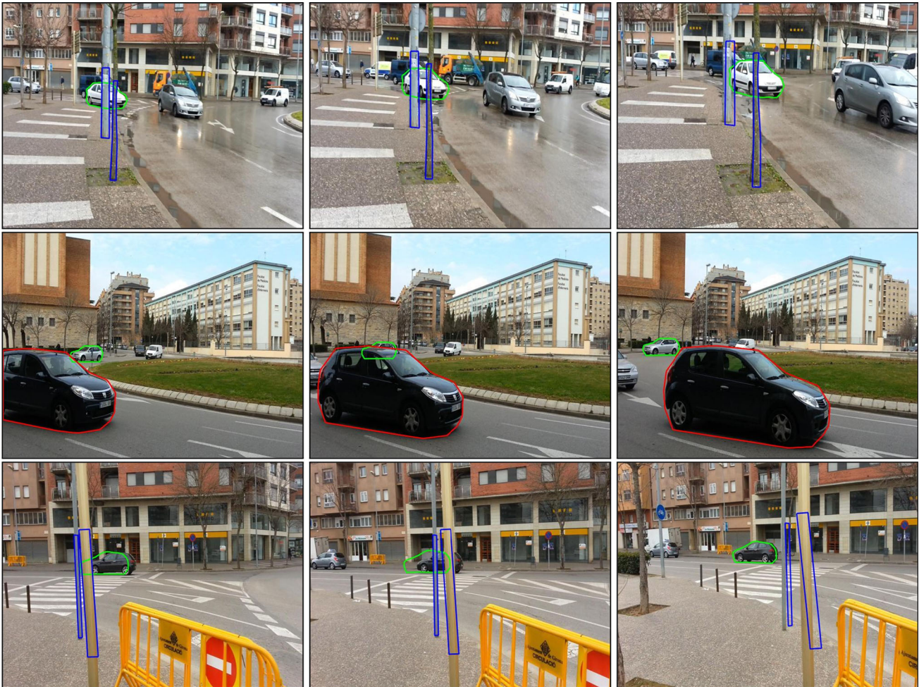
Fig. 10 Motion annotation result on three frames of three sequences is shown. The motion mask is shown in green contours. The static occluder masks are shown in blue, while the moving occluder mask is shown in red, contours. Top row: Frame 2, 18 and 37 from the sequence seq-19 . The moving white car is occluded by two static occluders, a lamp
