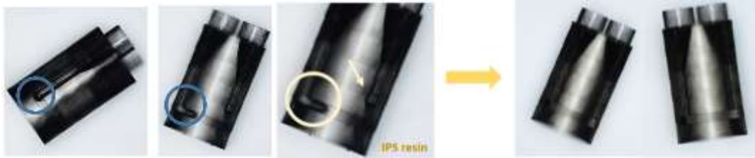
FIGURE 35: DEVICES WITH REMAINING RESIN INSIDE AND DEVICES WHEN IT HAS BEEN VANISHED (SONICATION)
