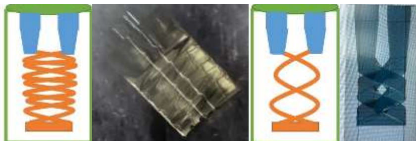
FIGURE 36: ON THE LEFT THE FIRST HELIX STRUCTURE AND ON THE RIGHT THE FINAL ONE (BIGGER ANGLES)
