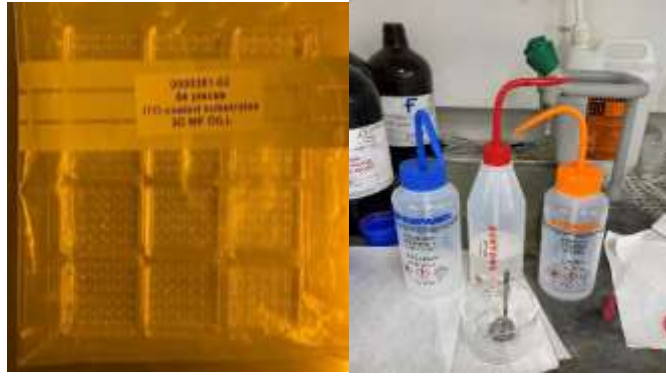
FIGURE 14: SUBSTRATES AND CHEMICALS USED (ITO-COATED SUBSTRATES 3D MF DILL AND ACETONE AND ISOPROPANOL)
