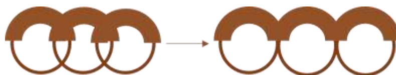
FIGURE 31: THE HIGHER THE HATCHING DISTANCE, THE LESS OVERLAP BETWEEN EACH VOXEL AND THE DARKER IT LOOKS
