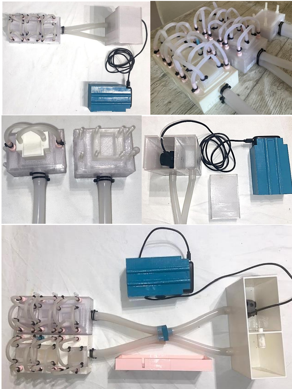
Figure 1. Final results. Images depict: (1,2) Assembly of the circuit in bioreactor mode; (3) individual culture channels module; (4) individual tank, lid, pump, and battery; and (5) assembly of the circuit in bioreactor mode utilising two channels modules and the extended tank.
