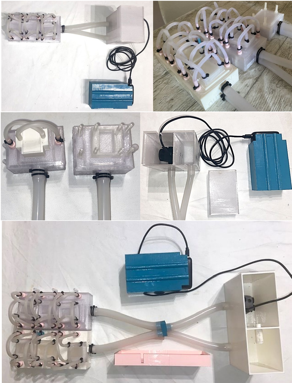
Figure 48. Final results. Images depict: (1,2) Assembly of the circuit in bioreactor mode; (3) individual culture channels module; (4) individual tank, lid, pump, and battery; and (5) assembly of the circuit in bioreactor mode utilising two channels modules and the extended tank.
