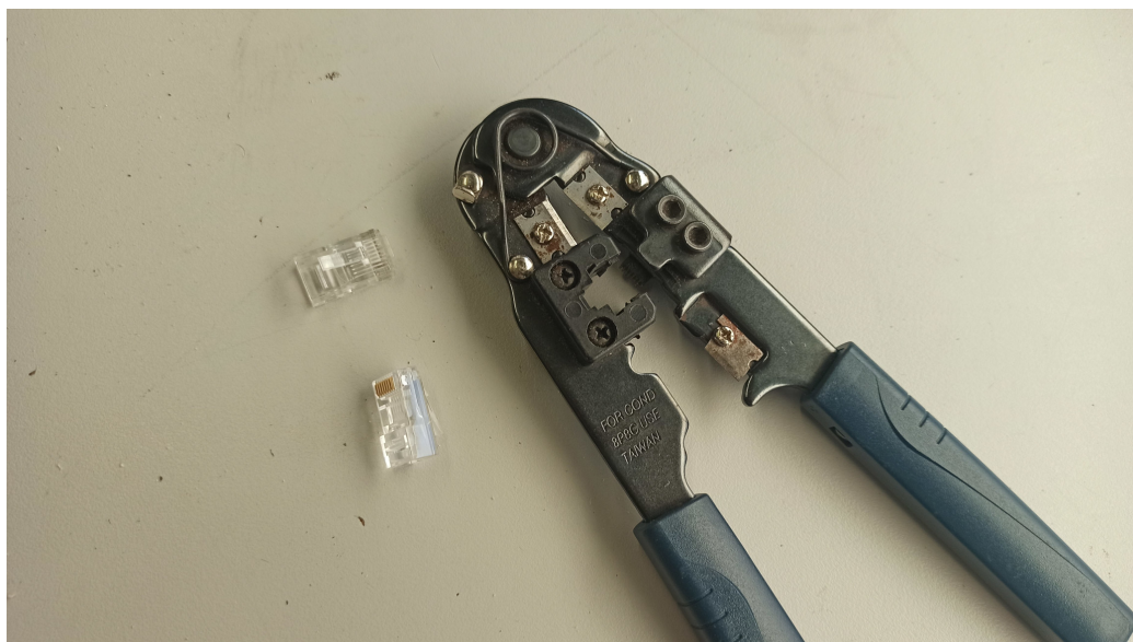
Figura 50: Connectors RJ45 i alicates per premsar-los
