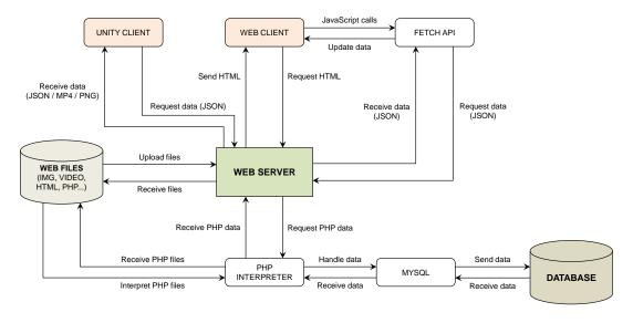
Figure 7: Client-server architecture of the TAECon platform.
