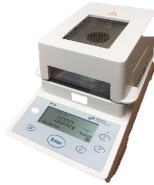
Figure 18: IDM IR-35 humidity analyser from Denver Instrument.
