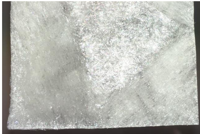
Figure 45: TEMPO aerogel at 0,3% of CNF consistency with some fibre orientation.
