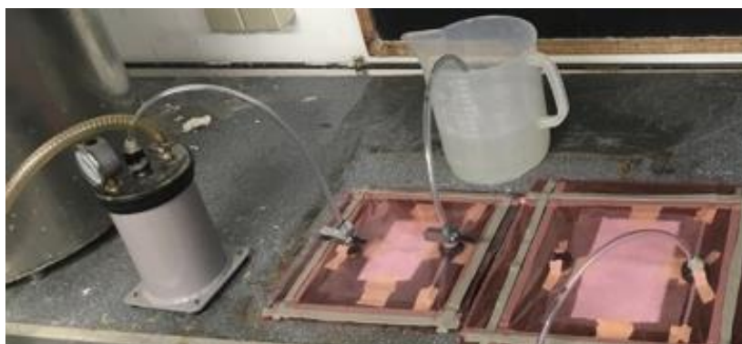
Figure 26: Real aspect of the final infusion assembly.
