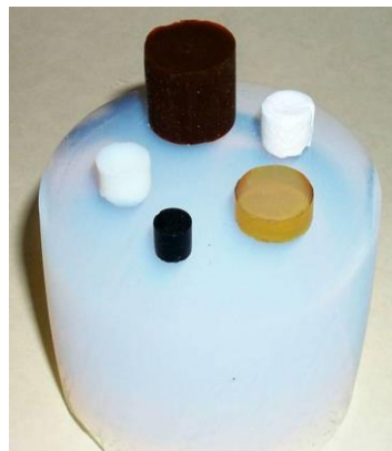
Figure 13: Transition metal oxide aerogels including an iron oxide (rust) aerogel (top). Source: Aerogel.org
