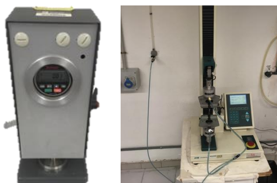
Figure 31: On the left the Starrett thickness gauge and on the right the Hounsfield dynamometer used to perform the stress-strain curves.
