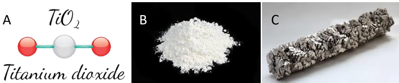
Figure 14: (A) Schematic representation of a Titanium dioxide molecule. (B) Titanium dioxide in the form of whitish powder, commercial form. (C) A titanium crystal bar, high purity 99,99%. Sources: 123RF Limited, 2019; Amazon.in, 2018.
