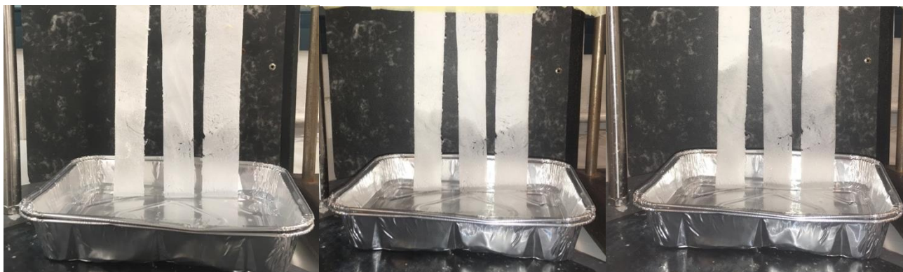
Figure 30: Water evolution by capillarity during the VWT.
