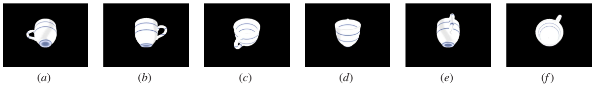
Figure 4: The six most representative views of the coffeecup object selected by the VMI algorithm.
