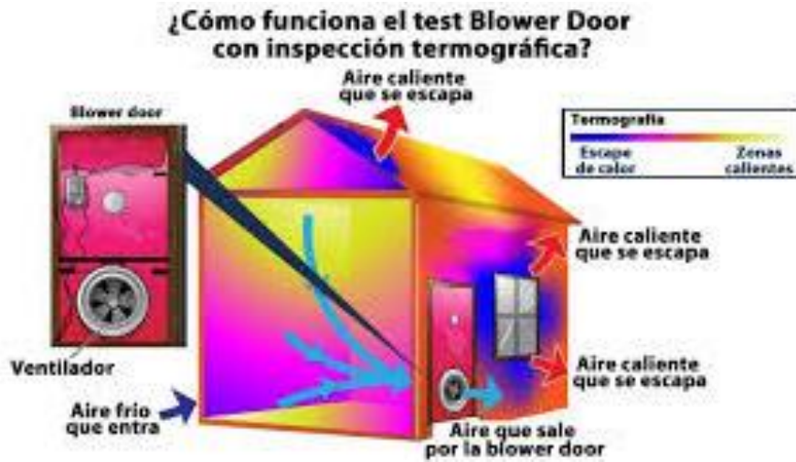
Figura 17: Test Blower Door. Font: https://www.facebook.com/linduxenergia/posts/745903215510212/
