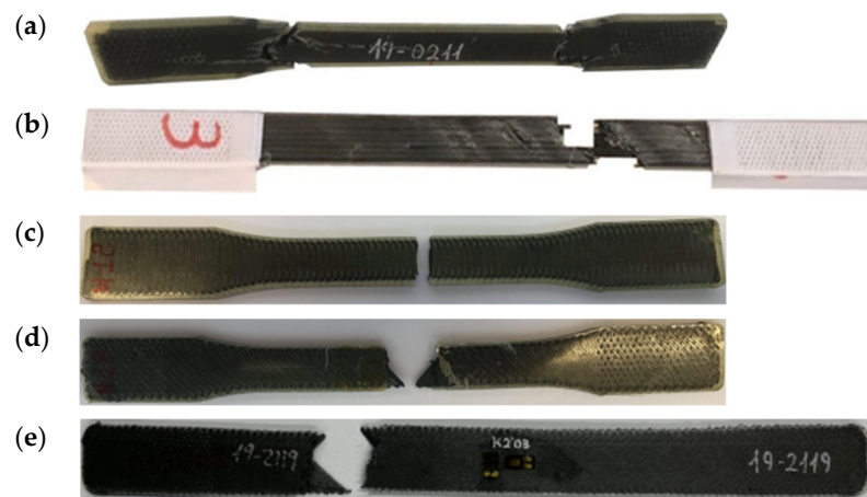
Figure 11. Representative failure type for each in-plane specimen configuration: (a) longitudinal ASTM D638 with failure at both fillet areas, (b) longitudinal ASTM D3039 with paper end-tabs with lateral failure in the gauge length, (c) transverse ASTM D638 with lateral failure, (d) in-plane shear ASTM D638 with typical \pm 45^\circ failure and (e) in-plane shear ASTM D3039 with typical \pm 45^\circ failure.
