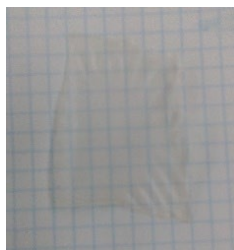
Figure 1. Kraft pulp cellulose films crosslinked with epoxides.
