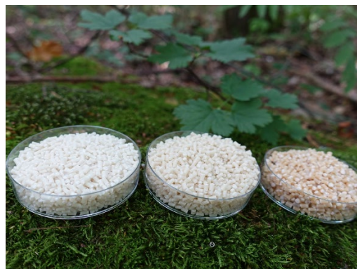
Figure 1. 3D-printable cellulose-based composite material
