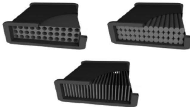
Figura 9: Estructures ordenades. Font: (Kitanovski, Energy application of magnetocaloric materials, 2020)
