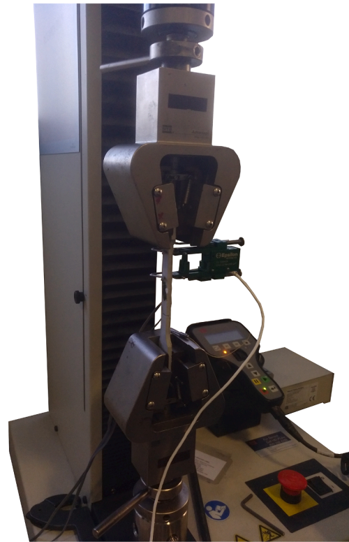
Fig. 1. Set-up for the instantaneous tensile test of adhesive specimens.
