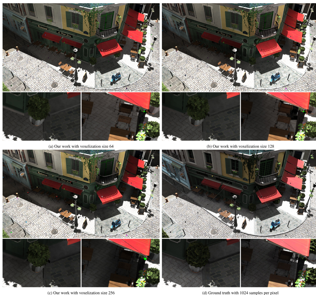
Fig. 16. In (a), (b) and (c) we show how, as voxelization size increases, the quality offered by our work gets closer to the ground truth, rendered in (d) with Cycles renderer (Blender v2.83) with 1024 samples per pixel. The 256 voxelization size case shows great similarities with the ground truth render, reproducing occlusion effects that are not present in renders with lower voxelizations. This is especially visible around the chairs and tables (see detail images). The peak signal-to-noise ratio values for our work at voxelization sizes 64, 128 and 256 and the ground truth render are 18.172, 18.203 and 17.42 respectively.
