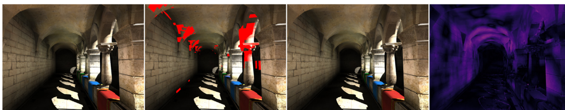
Fig. 9. From left to right: Sponza Atrium scene at a voxelization of size 256 (leftmost), showing in red the voxels that have not been assigned to any cluster (center-left). We added an extra pass to assign all unassigned voxels to its nearest cluster (center-right). A difference between the scene where not all voxels are assigned to a cluster (leftmost) and the scene where all voxels have been assigned to a cluster (center-right), generated using NVIDIA's FLIP [53] tool. As we can see in the leftmost image, taking into consideration all scene voxels as sources of irradiance for light gathering represents a small contribution in the final results for this scene and this voxelization size, which has the highest number of unassigned voxels to clusters (around 10%).
