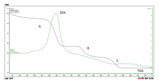
Figure 3. TG/DTA curves of the powder precursor of LaCrO<sub>3</sub>.
