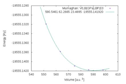
Figure 2. Total energy (Ry) vs. unit cell volume for LaCrO<sub>3</sub>H<sub>6</sub>.
