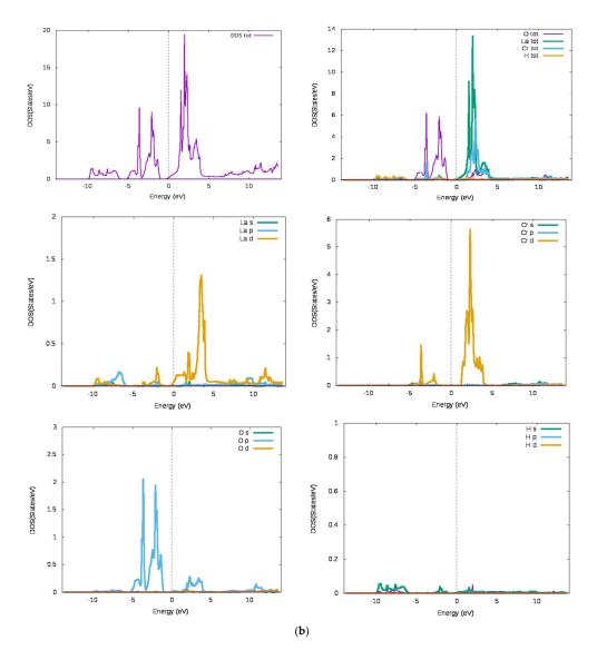
**Figure 1.** (a) Representation of the total and partial density of states of LaCrO<sub>3</sub>. (b). Total and partial density of states of LaCrO<sub>3</sub>H<sub>6</sub>.
