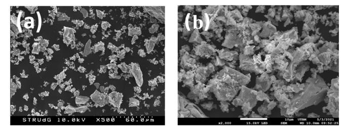
**Figure 5.** Field Emission Scanning Electron Micrographs of LaCrO<sub>3</sub> before and after hydrogenation (**a**,**b**) respectively.
