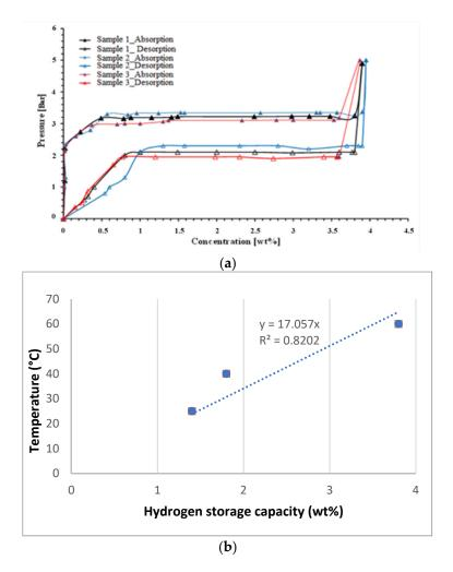
Figure 7. (a) PCT Curves of LaCrO<sub>3</sub> at 333 K, (b) Evolution of hydrogen storage with temperature.
