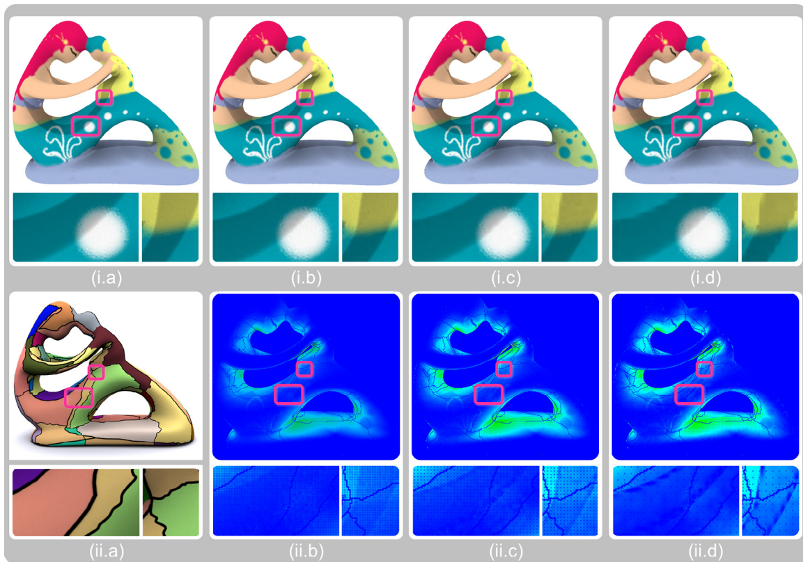
Fig. 9. Quality depending on the number of passes. Top row, from left to right: Ray-Casting reference and 2, 3 and 4 passes respectively. Bottom row: the clusters and the respective error images, computed with the L^2 metric, which show the increased error with the number of passes. The insets show details of the texturing and soft shadows. Timings are shown in Fig. 15.
