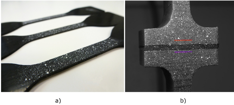
Fig. 6. (a) The prepared dumbbell specimens for the application of the DIC technique and (b) the DIC analysis on the butt-squared joint tensile tests.
