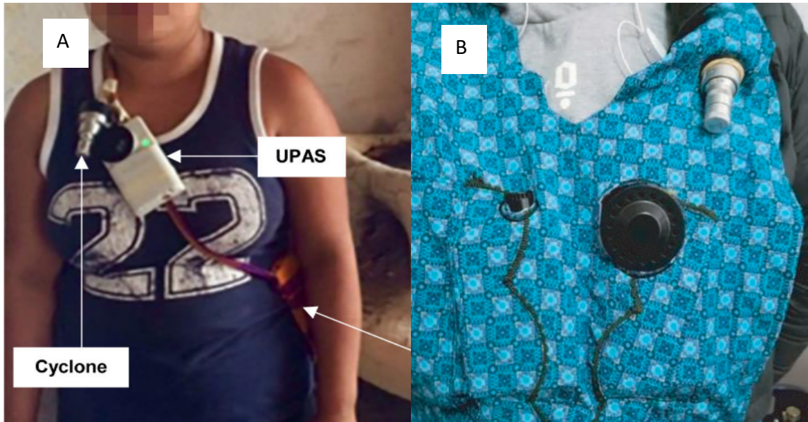
Figure 11: Participants of other studies wearing the UPAS device together with other monitors. A) The UPAS is the white monitor on the patient's chest (36). B) The patient has cut a whole on her clothes to expose the UPAS inlet (35)
