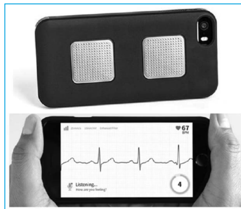
FIGURE 6: Top panel shows the AliveCor® case on a smartphone with both metal electrodes. The bottom panel shows a rhythm strip recorded by a user (39).
