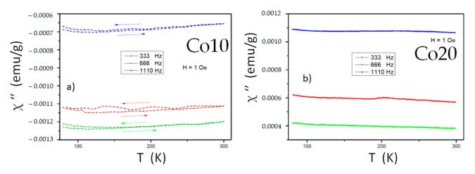
**Figure 8.** Magnetic susceptibility (imaginary component) of both alloys milled for 80 h (at different frequencies): (**a**) alloy Co10, (**b**) alloy Co20.
