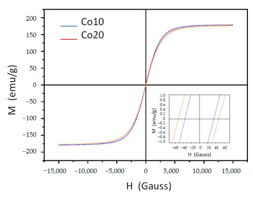
**Figure 6.** Magnetic hysteresis loops of both alloys milled for 80 h. The inset corresponds to the (0, 0) area.
