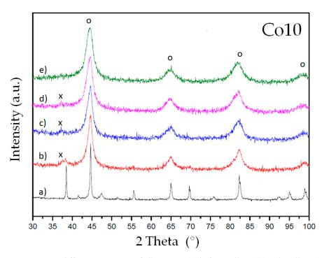
**Figure 1.** XRD diffraction patterns of alloy Co10: (**a**) before milling, (**b**) 10 h milling, (**c**) 20 h milling, (**d**) 40 h milling and (**e**) 80 h milling. Symbols: o marks the bcc reflections of the main phase and x marks the main reflection of a Nb(B) phase.
