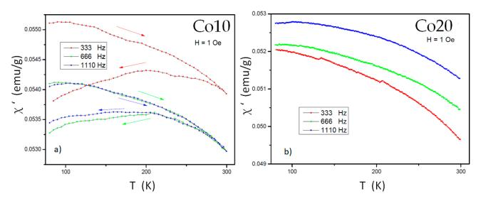
**Figure 7.** Magnetic susceptibility (real component) of both alloys milled for 80 h (at different frequencies: (**a**) alloy Co10, (**b**) alloy Co20.
