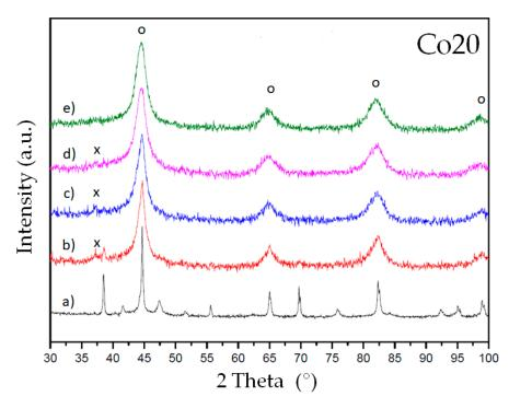
**Figure 2.** XRD diffraction patterns of alloy Co20: (**a**) before milling, (**b**) 10 h milling, (**c**) 20 h milling, (**d**) 40h milling and (**e**) 80 h milling. Symbols: o marks the bcc reflections of the main phase and x marks the main reflection of a Nb(B) phase.
