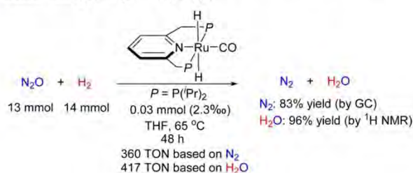
Scheme 1. Hydrogenation of N 2 O by the PNP-pincer Ru based catalyst 1 (P = P(iPr) 2 )
