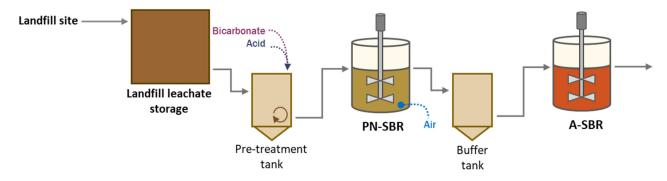
Figure 1. Descriptive scheme for the PANAMMOX<sup>®</sup> technology.
