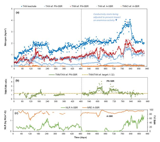
**Figure 6.** Performance of the full-scale system at the long-term; (**a**) Evolution of the concentration of the N species in both reactors (TAN: total ammonium N, TNN: total nitrite N, TNNO: TNN+ nitrate N); (**b**) TNN/TAN ratio in the PN-SBR effluent; (**c**) N loading rate and removal efficiency in A-SBR. Day 0 is 1 September 2017. The vertical dashed lines indicate when the landfill site stop receiving solid waste (on day 486).
