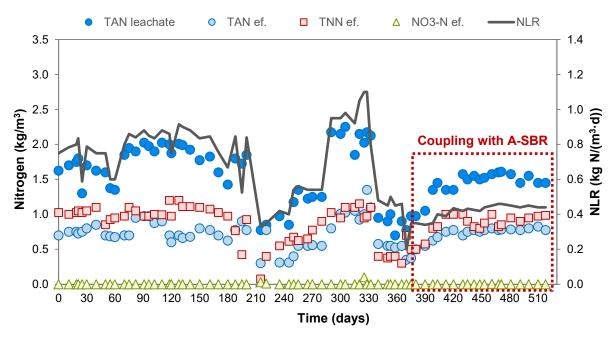
**Figure 3.** Long-term performance of the pilot-scale PN-SBR treating raw landfill leachate. By the end of the running period, PN-SBR was coupled with A-SBR (see Figure 4, *PHASE II-c*).
