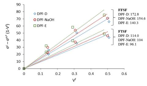
Figure 9. Fiber tensile strength factor and fiber flexural strength factor of date palm fiber composites.
