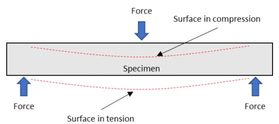
Figure 8. Compression and tensile force combination during the flexural test.
