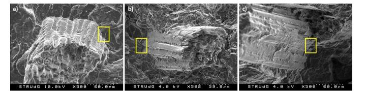
**Figure 6.** SEM micrograph of the flexural fractured surface for (**a**) mechanical pretreated date palm fibers; (**b**) chemical pretreated date palm fibers; (**c**) enzymatic pretreated date palm fibers.
