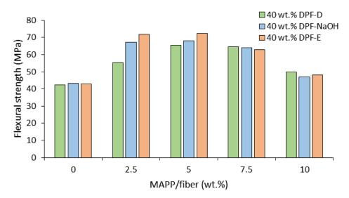
**Figure 5.** Effect of coupling agent concentration on composites loaded with a 40 wt.% of date palm fibers.
