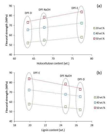
**Figure 7.** Evolution of the flexural strength of composites with the holocellulose (**a**) and lignin content (**b**).
