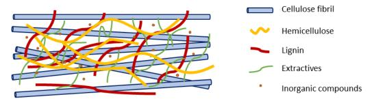
Figure 4. Illustration of the main chemical constituents in the fiber cell wall.
