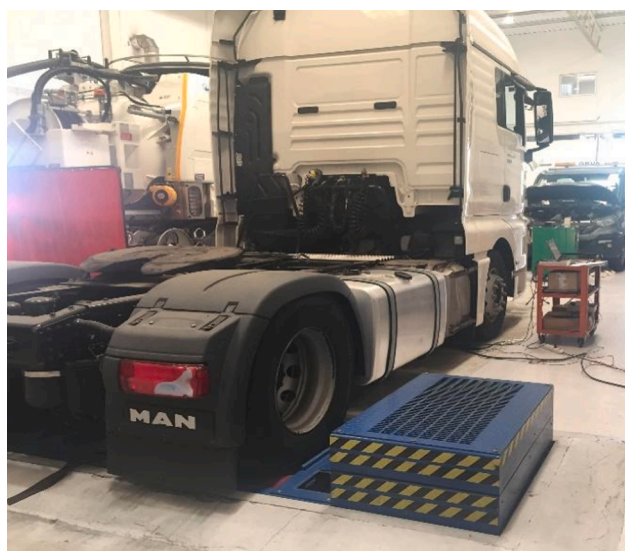
Fig. 7. Vehicle position on the rolling bench during the experiment.
