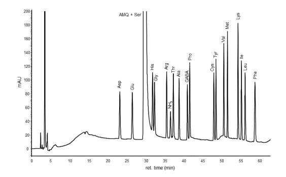
Figure 2. Chromatogram obtained in the analysis of a calibration solution at 100  $\mu$ M level prepared from the 17 AA standard solution.
