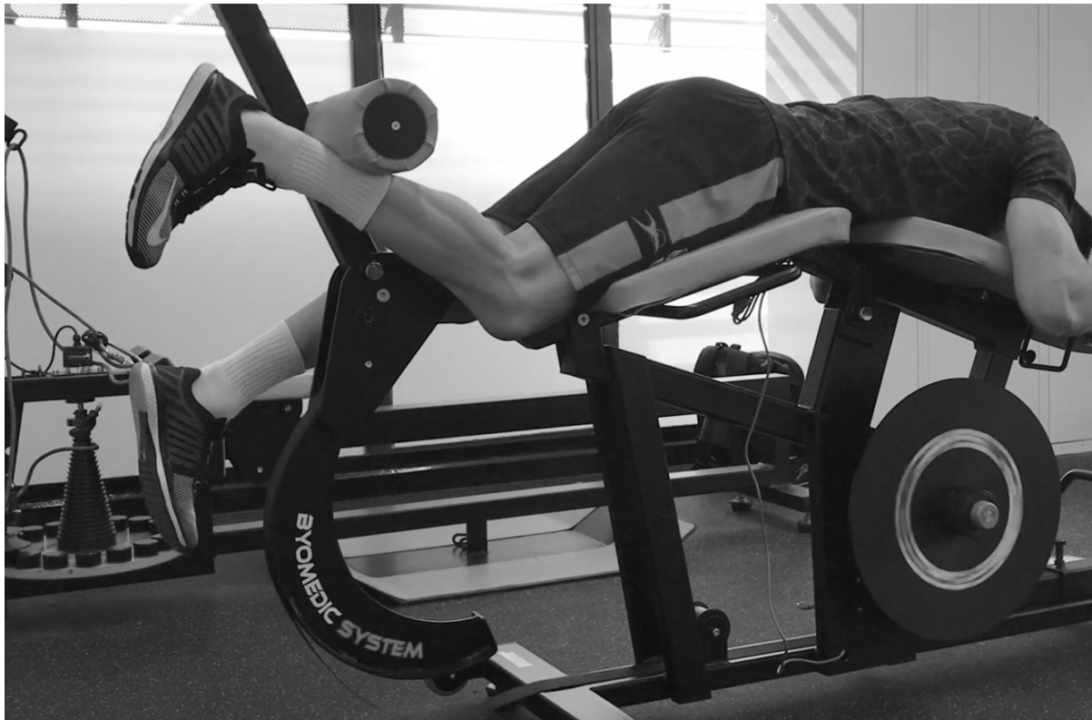
Figure 9. Leg-curl with a flywheel iso-inertial device.
