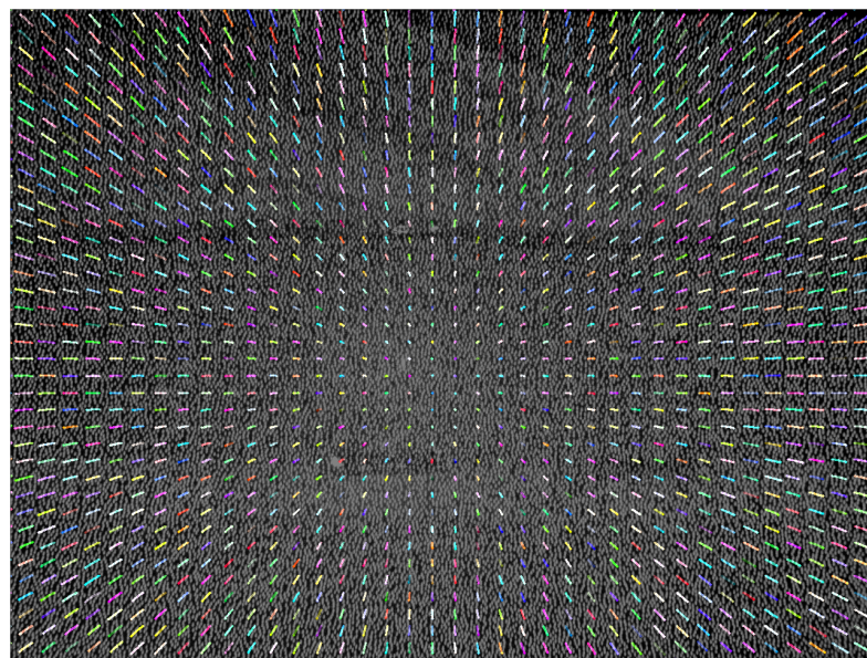
Figure 4. Expansion of the captured IR pattern with the temperature using the optical flow algorithm.
