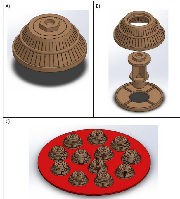
Figure 1.13. Inserted domes underdrain design. A) Dome, B) Dome interior design, C) Inserted dome underdrain. Source: Bové (2018).
