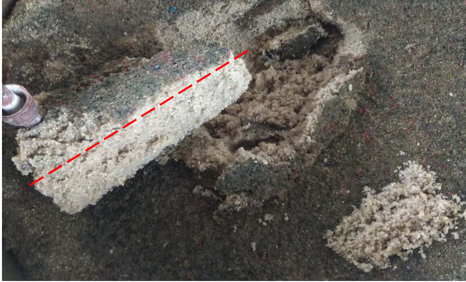
Figure 6.9. Debris deposition in the firsts centimetres (dotted line) on the first media layer after 250 h of filtration with 0.3 m and 30 m/h for porous media design.
