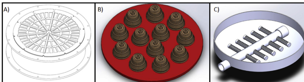
Fig. 1 – Different underdrain designs: porous media (A), inserted domes (B) and arm collector (C).
